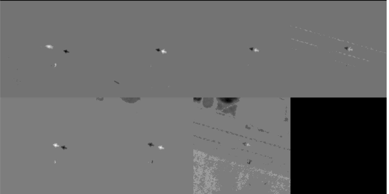
**Figure 6.** Same as figure 5 after thresholding the images at a constant level based on the histogram of image brightness levels. The same threshold has been applied to all images.
