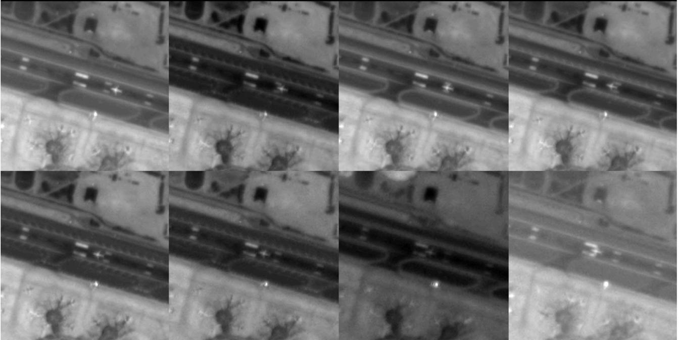
**Figure 4.** Detail of the full image in eight spectral bands arranged in temporal order: top row, right-to-left, then bottom row, right-to-left. In this temporal order showing the airplane moving west (left), the spectral bands are B, R, G1, G2, Y, RE, NIR, CB (table 1). Each panel covers  $0.6 \times 0.6$  km.
