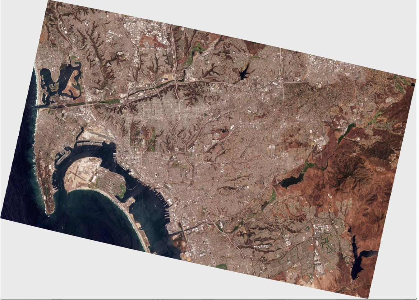
**Figure 1.** Composite visual image from the Planet Labs data set 20220530\_173806\_19\_241e. The image contains  $13317 \times 9578$  pixels of  $3 \text{ m}^2$  covering  $40.0 \times 29.7 \text{ km}^2$  including the regions with no data.
