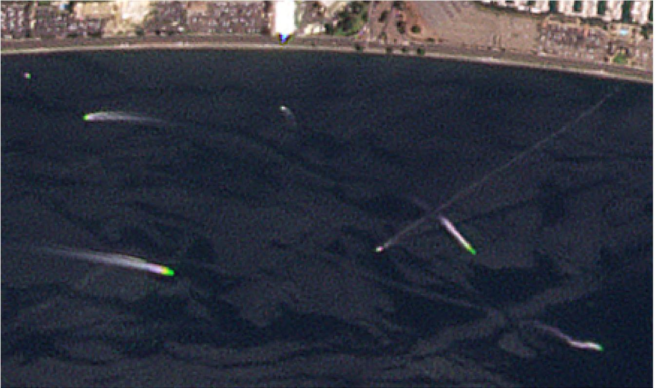
**Figure 3.** Detail of the composite visual image (figure 1) showing boats moving in the San Diego harbor. The bright green leading edge is a characteristic signature of motion. The image covers  $1.31 \times 0.78$  km.
