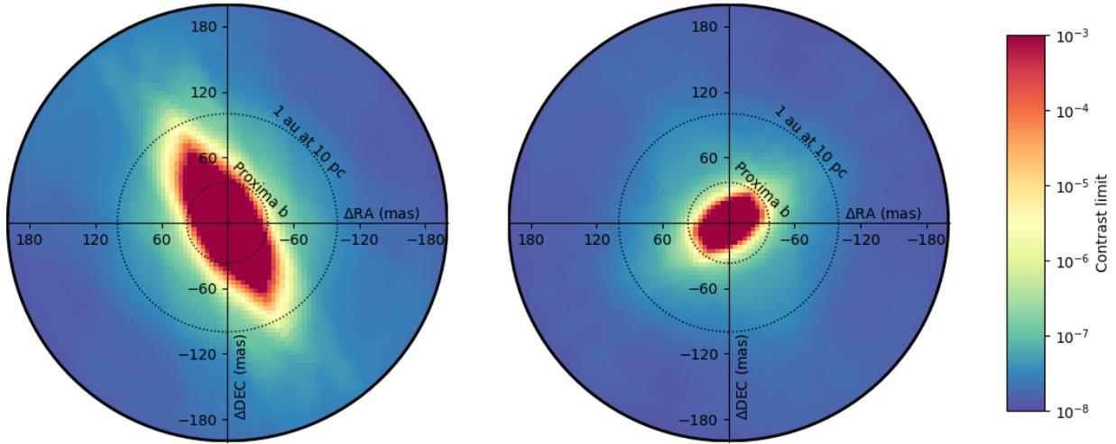
**Fig. 8.** Contrast limit of a dual-field interferometer using the current four-UT configuration of the VLTI, compared to the proposed five-UT configuration shown in Figure 9.
