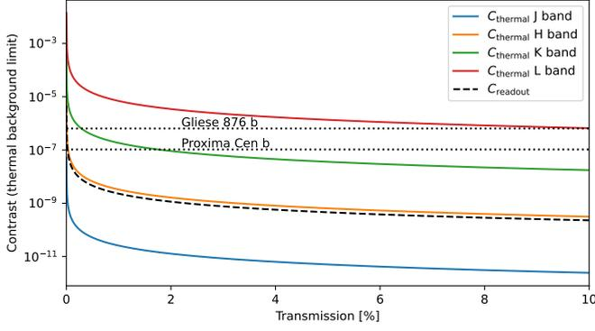
**Fig. 2.** Contrast limit at the VLTI as a function of the total transmission of the interferometer. The coloured curves represent theoretical contrast limits set by the thermal background of the telescope and interferometric laboratory (300 K). The dashed curves indicate the contrast limit from detector readout noise. The simulation parameters are detailed in Table 2.
