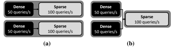
Fig. 4: An example RecSys where the dense DNN layer exhibits half the QPS than the sparse embedding layer. (a) How the baseline model-wise resource allocation would replicate two servers to reach 100 queries/sec and (b) how our proposed ElasticRec would reach such QPS goal using fine-grained, per-layer resource allocation.
