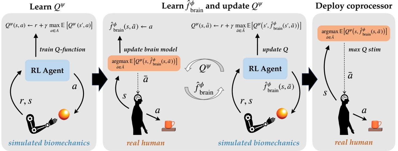
Figure 1. Overview of our framework. We first learn the Q-function,  $Q^\psi$ , for world actions,  $a$ , via a biomechanically realistic simulator. We then learn the mapping,  $\hat{F}_{\text{brain}}^\phi$ , from coprocessor actions,  $\bar{a}$ , to world actions. Simultaneously, we update  $Q^\psi$  to account for the altered MDP.
