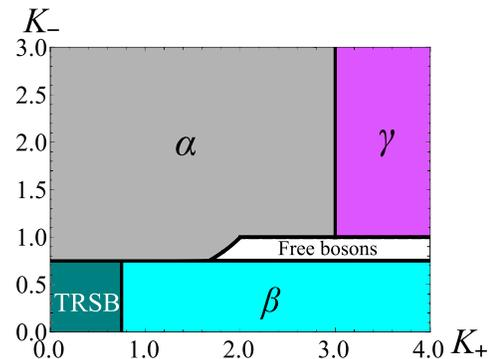
FIG. 3. Generic phase diagram for  $n = 1$ . We consider a weak Rashba spin-orbit coupling such that the total  $S_z$  is approximately conserved. The TRSB and  $\alpha$  phases are insulating. The free bosons,  $\beta$ , and  $\gamma$  phases give conductance  $G = 2 \frac{e^2}{h}$ .
