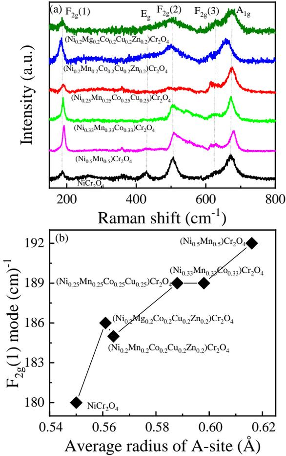
FIG. 6. (a) Raman spectra for all the materials collected at room temperature. (b) Shift of the  $F_{2g}(1)$  mode with the variation of the radius of the A site for all the samples.
