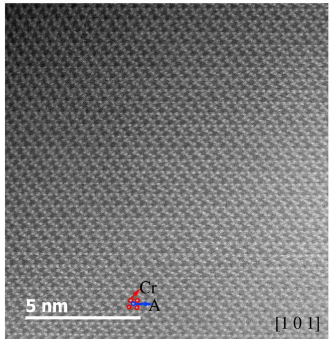
FIG. 5. STEM - HAADF image along the [101] zone axis for  $[\text{Ni}_{0.2}\text{Mg}_{0.2}\text{Co}_{0.2}\text{Cu}_{0.2}\text{Zn}_{0.2}]\text{Cr}_2\text{O}_4$ , collected at room temperature. Cr and A site cations are shown in the figure.
