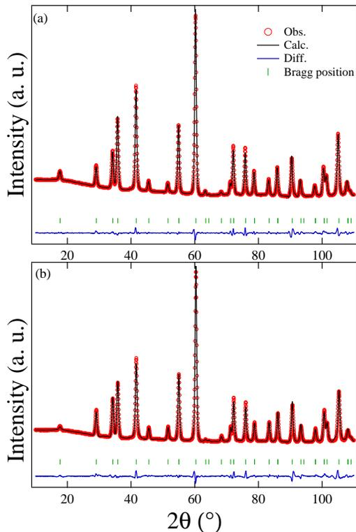
FIG. 4. Rietveld refinement plots of the room temperature neutron powder diffraction (NPD) patterns for (a)  $[\text{Ni}_{0.2}\text{Mn}_{0.2}\text{Co}_{0.2}\text{Cu}_{0.2}\text{Zn}_{0.2}]\text{Cr}_2\text{O}_4$  and (b)  $[\text{Ni}_{0.2}\text{Mg}_{0.2}\text{Co}_{0.2}\text{Cu}_{0.2}\text{Zn}_{0.2}]\text{Cr}_2\text{O}_4$ .
