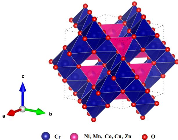
FIG. 1. Crystal structure of the spinel  $AB_2O_4$  oxides. B cations (here Cr) occupy the octahedral sites, A cations (Ni, Mn, Mg, Co, Cu, Zn) occupy the tetrahedral sites
