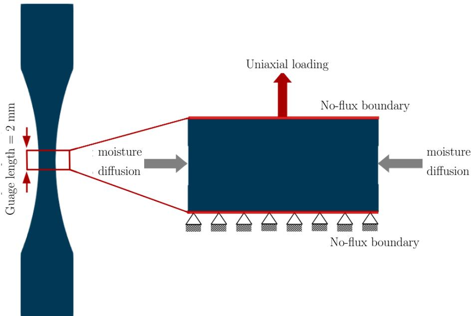
Figure 8: Left and right faces of 2 mm wide cross-section of the tailored tensile sample is subject to moisture diffusion for time  $t$  s with no-flux boundaries and then the sample is uniaxially loaded with a strain rate of  $0.0005 \text{ s}^{-1}$
