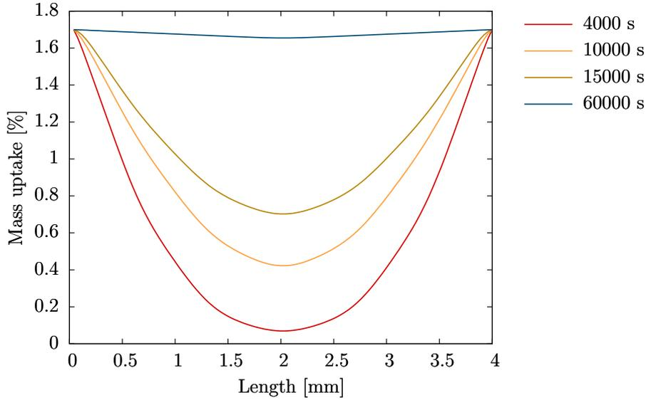
Figure 9: Distribution of moisture over the cross-section of the adhesive sample determined by simulation at different times
