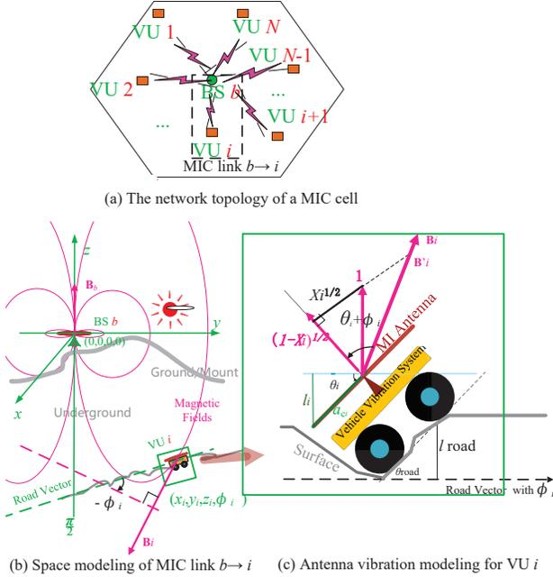
Fig. 1. Antenna vibration modeling for the channel from BS  $b$  to VU  $i$ ,  $\theta_i \in [-90^\circ, 90^\circ]$  is the angle of the antenna vibration,  $\phi \in [-180^\circ, 180^\circ]$  represents the antenna background orientation,  $X_i$  is the AVI.
