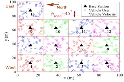
Fig. 10. A CVMC network for CVMC-PCO simulations where  $z_{\text{west}}=10\text{m}$  (see Fig. 3),  $\phi_{\text{road}}\simeq 45^\circ$ ,  $K=13$  and  $N=32$ . Each VU moves in a random walk with the maximal velocity of 2m/s. Its average AVI  $\sigma_{[k,n]}^2$  varies randomly at the end of every time  $25t$ .
