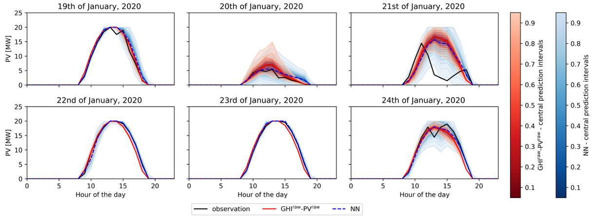
Figure 7: Exemplary probabilistic PV forecasts for dates in January 2020 for  $\text{GHI}^{\text{raw}}\text{-PV}^{\text{raw}}$  and  $\text{GHI}^{\text{PP}}\text{-PV}^{\text{PP}}$  with the NN jointly estimated for all hours of the day. The colored areas indicate central prediction intervals. The lines show the ensemble median.
