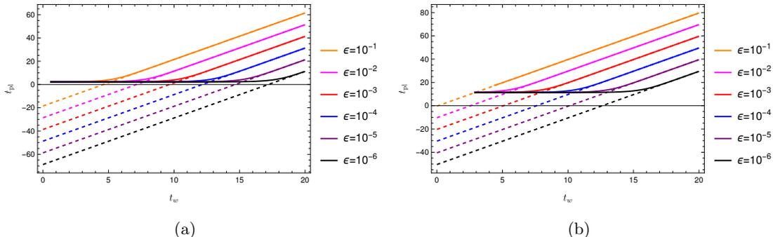
**Figure 14:** Duration of the plateau regime (3.24) as a function of the insertion time of the shockwave, for various choices of  $\varepsilon$  defined in eq. (2.19) in  $d = 2$ . (a) We fix  $L = 1, \delta = 0.05, G_N \mathcal{E}_1 = 0.02$  and  $\rho = 0.5$ . The dotted lines corresponds to the curves  $t_{\text{pl}} = 4(t_w - t_*)$  with scrambling time in eq. (3.27). (b) Same plot, but using the parameter  $\rho = 0.99$  instead.
