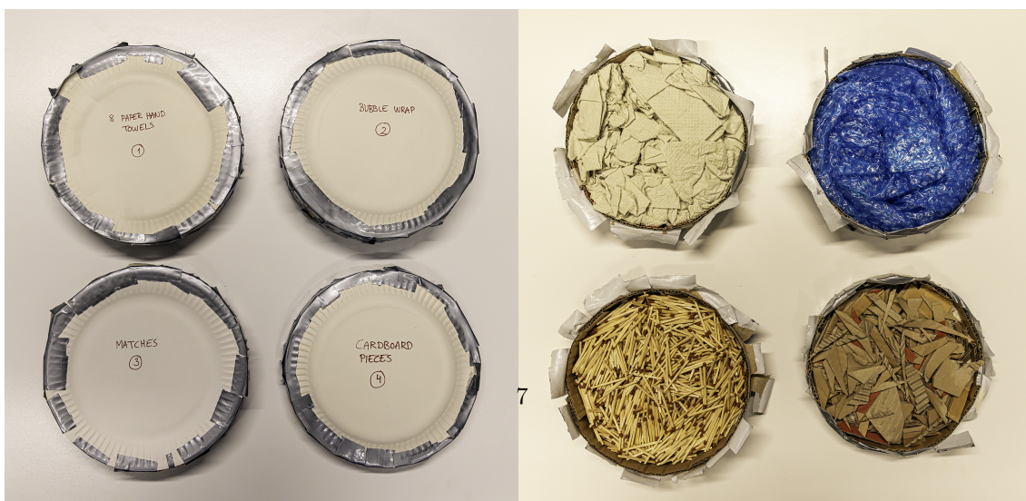
Figure 5: Discs made out of two paper plates filled with different materials (paper towels, bubble wrap, matches, cardboard pieces) and taped together were also used between the speaker and microphone.
