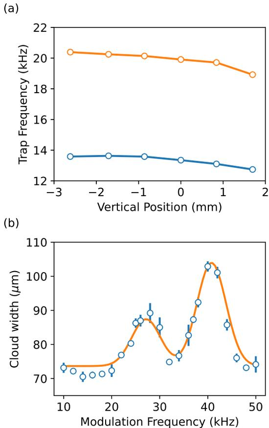
FIG. 5. (a) Transverse trap frequencies as a function of ODT position. (b) Typical modulation spectrum, showing cloud size (one standard deviation of the vertical density distribution) after 0.1 ms time-of-flight. The peaks correspond to 2 times the transverse trap frequencies.
