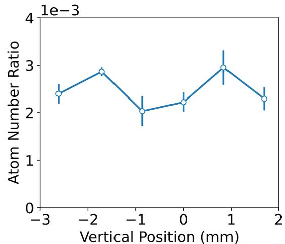
FIG. 4. Fraction of atoms transferred from gray molasses to the crossed ODT vs position of the ODT. The gray molasses is also moved to match the ODT location by adjusting the vertical bias field.
