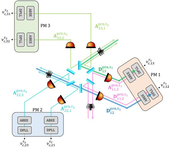
FIG. 4. A diagram of the PRNR protocol without bias correction. In this example, the interferometric signals at PM 2 and 3 and  $v_{c,13}^{\tau_1}$  at PM 1 are shifted to the readout time of  $v_{c,12}^{\tau_1}$  at PM 1. ABEE stands for analog back-end electronics.
