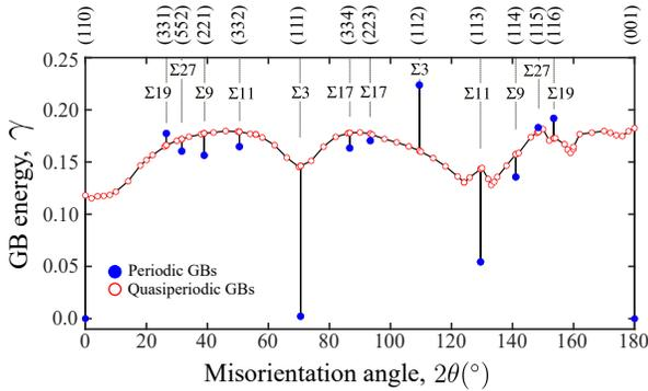
FIG. 5. GB energy as a function of misorientation angle for [110] symmetric tilt GBs. Periodic GBs are represented by blue solid circle, labeled with the  $\Sigma$  value and the boundary plane normal direction. Quasiperiodic GBs are indicated by red hollow circles.
