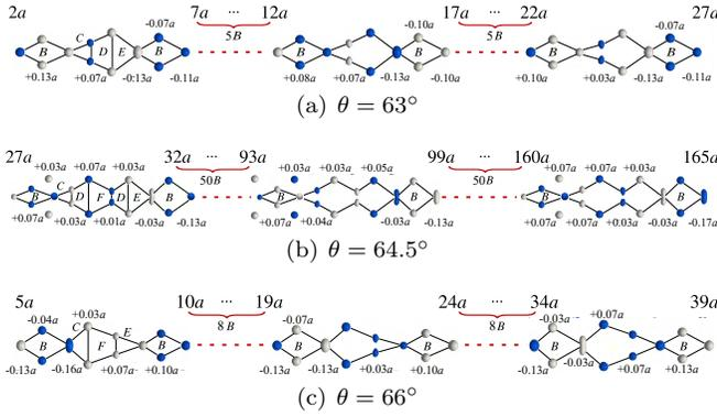
FIG. A.4. Quasiperiodic GBs with tilt angles (a)  $\theta = 63^\circ$ ; (b)  $\theta = 64.5^\circ$ ; (c)  $\theta = 66^\circ$ . Structural units and offsets are labeled. The omitted parts are duplicate structural units  $B$ .
