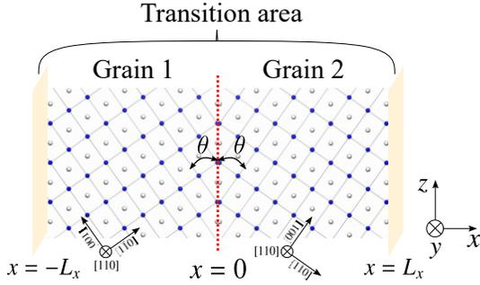
FIG. A.1. The schematic of  $[110]$  symmetric tilt GBs in FCC.  $\theta$  is the tilt angle.
