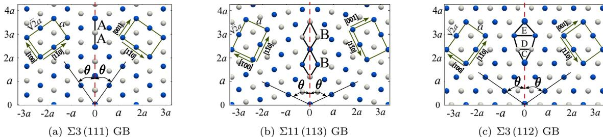
FIG. 1. Periodic GBs: (a)  $\Sigma 3(111)$  GB; (b)  $\Sigma 11(113)$  GB; (c)  $\Sigma 3(112)$  GB. The red dashed line indicates the  $x = 0$  plane. Structural units on GBs are marked with solid black lines. Tilt angles, single cells and grain orientations are labeled.
