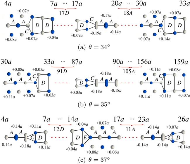
FIG. 3. Quasiperiodic GBs with tilt angles (a)  $\theta = 34^\circ$ ; (b)  $\theta = 35^\circ$ ; (c)  $\theta = 37^\circ$ . Displacements of spheres from bulk locations are labeled. The omitted region comprises a repetitive arrangement of structural units, either  $A$  or  $D$ .
