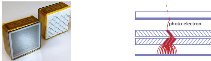
Fig. 3. The Hamamatsu R10754-07-M16(N) microchannel plate photomultiplier tube (left). Two microchannel plates with angled channels (right).
