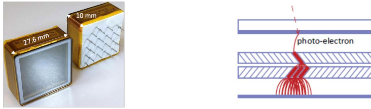
Fig. 3. The Hamamatsu R10754-07-M16(N) microchannel plate photomultiplier tube (left). Two microchannel plates with angled channels (right).
