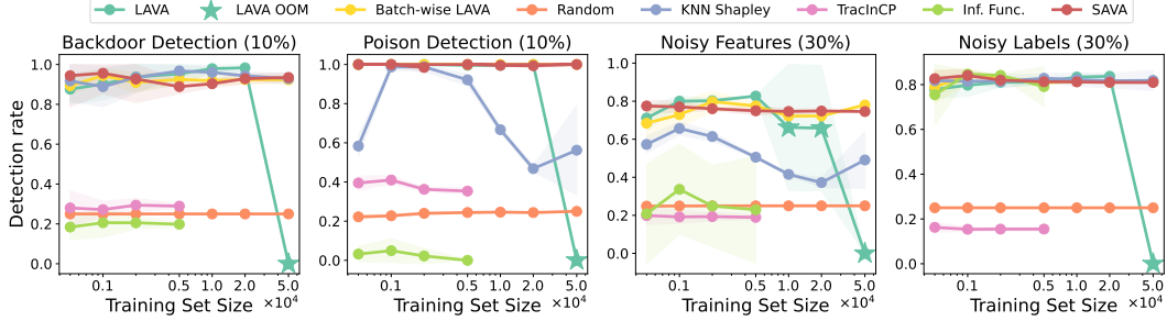
Figure 2: SAVA can value the full CIFAR10 dataset with various corruptions, while LAVA has out-of-memory (OOM) issues. We sort training examples by the highest OT gradients in Eq. (6) and Eq. (12) for LAVA and SAVA respectively, and use the fraction of corrupted data recovered for a prefix of size N/4 as the detection rate (where N is the training set size). The star symbol ( \star ) denotes the point at which LAVA is unable to continue valuing training due GPU out-of-memory (OOM) errors.
