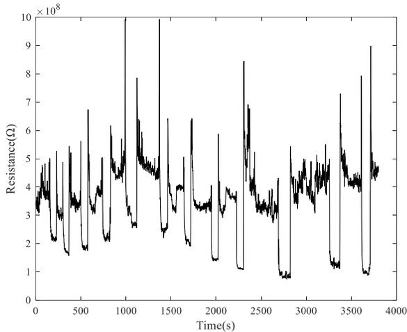
Fig. 3. Sensor concentration curve for acetone
