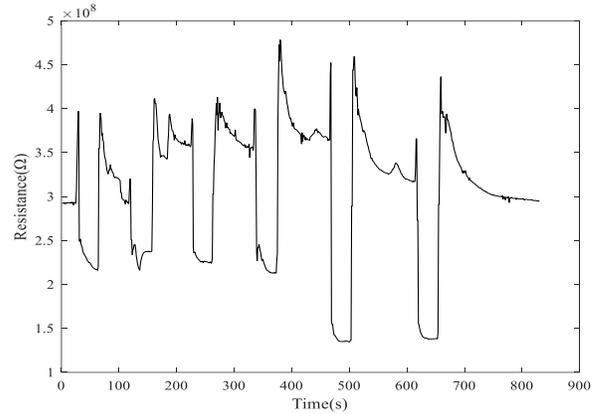
Fig. 5. Sensor concentration curve for methanol
