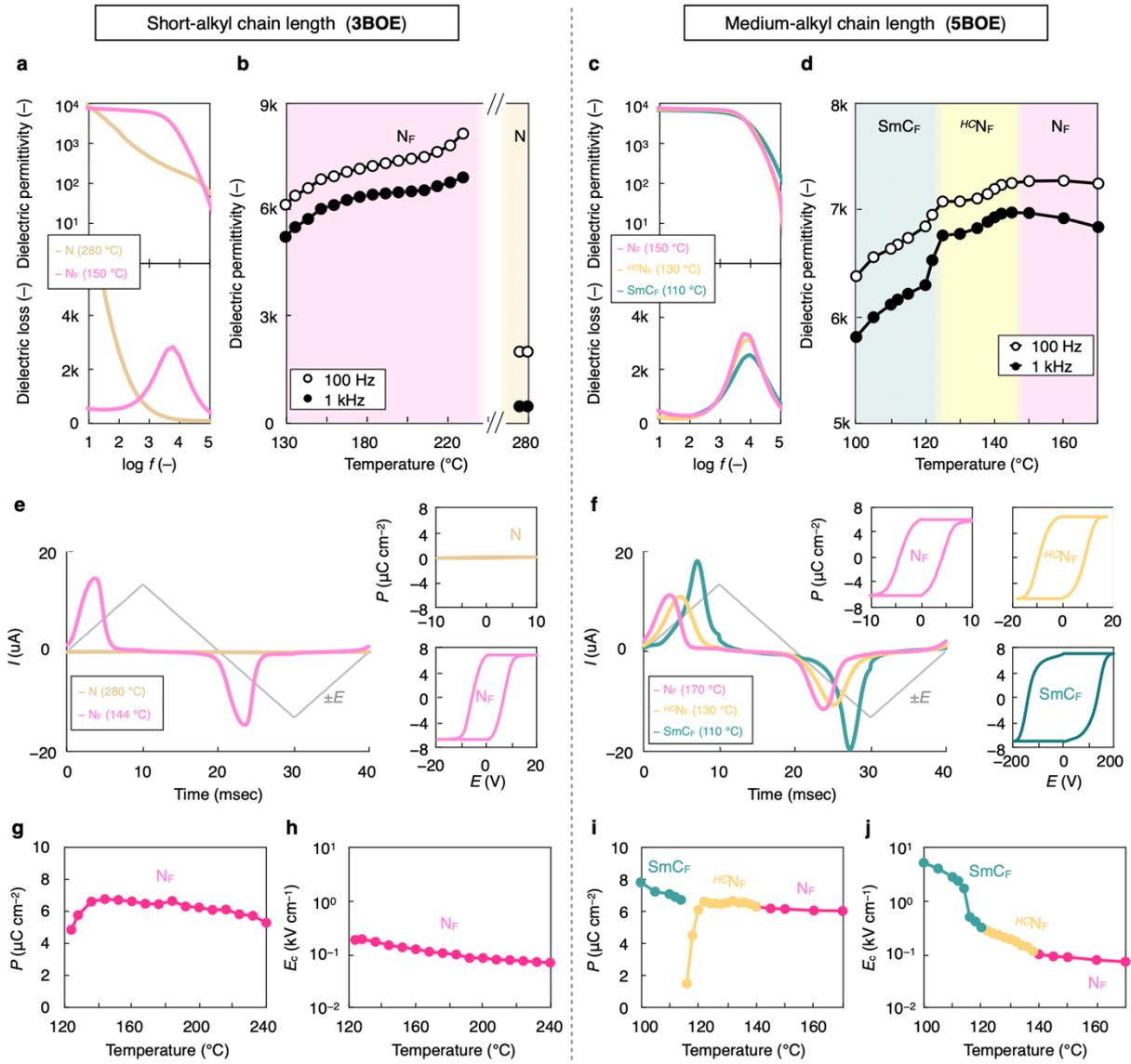
**Figure 3** Polarization behavior. Dielectric spectra (3BOE: a, 5BOE: c) and dielectric permittivity vs temperature (3BOE: b, 5BOE: d). Polarization reversal current profile (3BOE: e, 5BOE: f). Insets represent the corresponding  $P$ – $E$  hysteresis curves. Polarization density vs temperature (3BOE: g, 5BOE: i). Coercive electric field ( $E_c$ ) vs temperature (3BOE: h, 5BOE: j).
