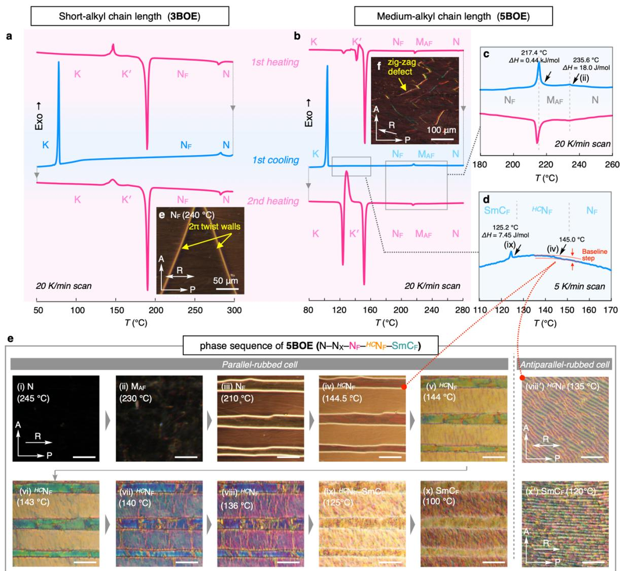
**Figure 2.** DSC studies. DSC curves of **3BOE** (a) and **5BOE** (b–d). Scan rate:  $20 \text{ K min}^{-1}$  (a,b,c),  $5 \text{ K min}^{-1}$  (d). e) POM images taken under cross polarizers in the parallel- and antiparallel rubbed cells. bar:  $50 \mu\text{m}$ . Areas designated by Roman numerals (i–x, viii' and x') corresponds to the observations in DSC and POM studies.
