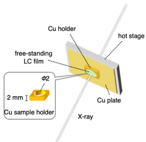
**Figure S2 Measurement setup for XRD studies.**
