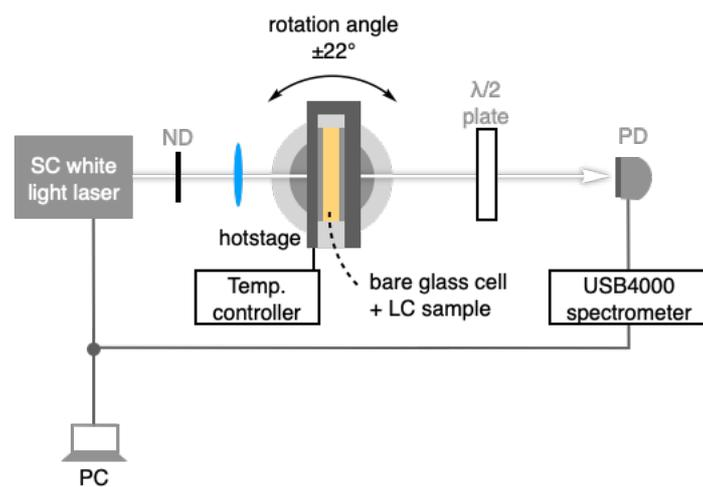
**Figure S3 Optical setup for Spectra studies. Cell thickness: 5  $\mu\text{m}$ .**
