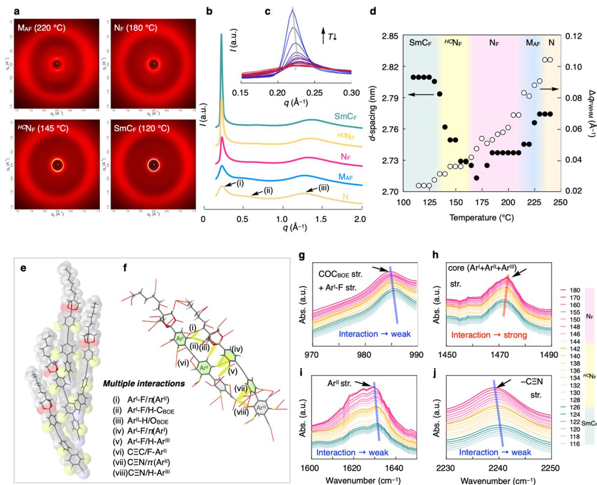
**Figure 4.** XRD and FTIR spectra studies. 2D XRD (a) and 1D XRD (b,c) pattern in various phases for **6BOE**. (d)  $d$ -spacing and FWHM vs Temperature for **6BOE**. Structures of local cluster (e) and adjacent dimer (f) extracted from SC-XRD data for **6BOE**. (g–j) FTIR absorbance spectra for **5BOE**. For the panel (b), the recorded temperature in N, N<sub>F</sub>, <sup>HC</sup>N<sub>F</sub> and SmC<sub>F</sub> phases are 240, 220, 180, 145 and 120 °C, respectively.
