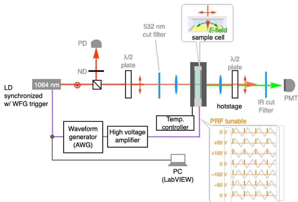
**Figure S1 Optical setup for SHG studies.** The electric field ( $E$ -field) was applied normally to the sample cell (thickness: 5  $\mu\text{m}$ ).
