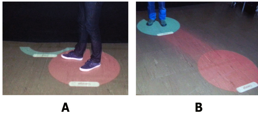
Fig. 6. Out of reach users: (A) While out of reach, a representation of the participant remains on the boundary of the local area. (B) Visual feedback on the projected floor shows an interaction request to the out of reach participant.
