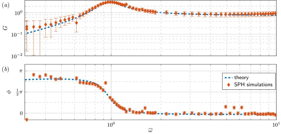
FIG. 5. **Gain and phase of the synchrotron water waveguide:** Results for  $\bar{\lambda} = 10$ . Comparison between SPH simulations (red diamonds) and analytical results using equation (2) (dashed blue line). Theoretical curves corresponds to  $\bar{\Theta} = 0.0958$  ( $\nu = 1.5$  cSt).
