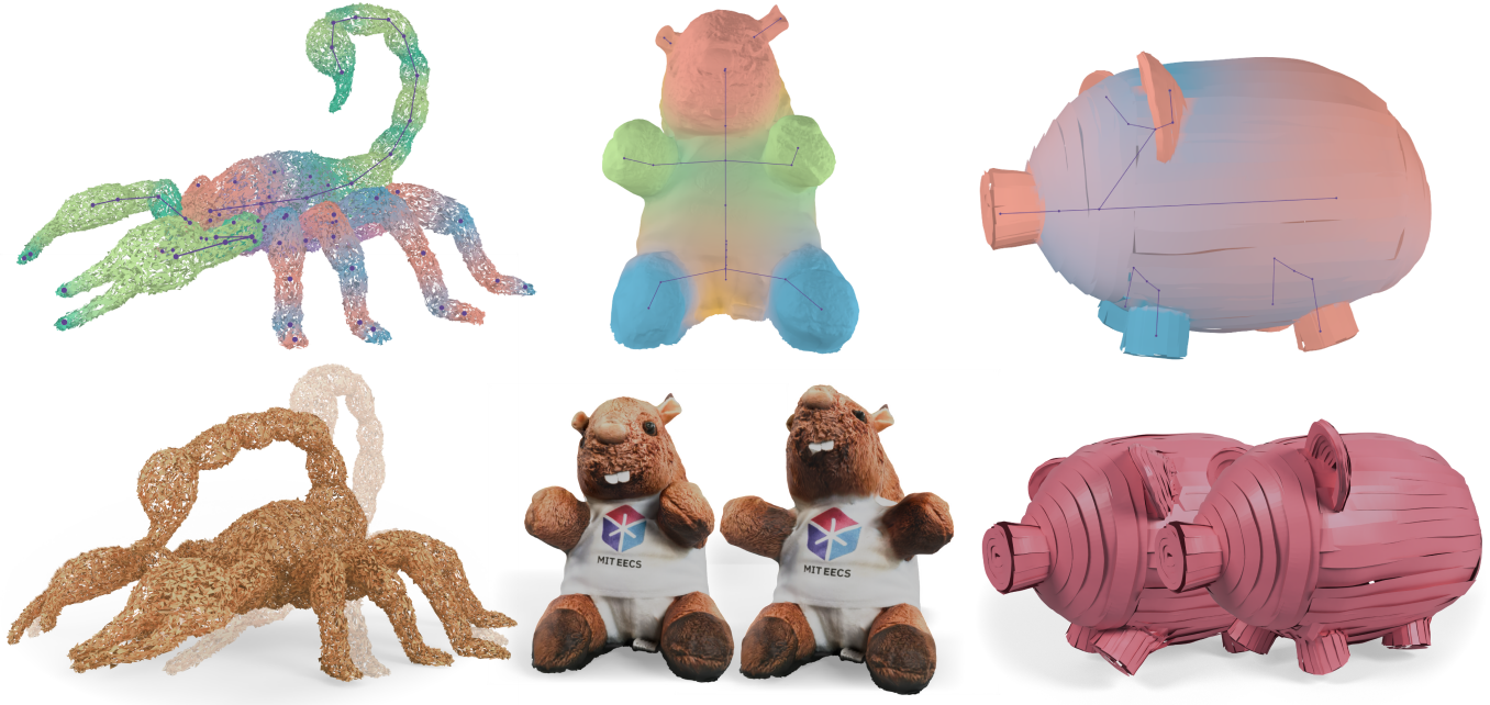
Fig. 1. Biharmonic skinning weights produced by our method can be used to extrapolate color (top row) or deformations (bottom row) from the control handles into the shape and onto its boundary. Our method computes biharmonic skinning weights on meshes that are typically difficult to handle with standard optimization methods. The SCORPION mesh has been heavily degraded by removing 30% of its faces and randomly perturbing the remaining ones. Our method can compute smooth skinning weights for the BEAVER mesh, created using off-the-shelf 3D scanning software (note: the center of the mesh has been blurred for anonymity). As a result, it contains many thin and self-intersecting triangles, a typical source of errors in finite element solvers. Our method can also be used to deform virtual reality ribbon drawings [Rosales et al. 2019], such as the PIGGYBANK mesh.
