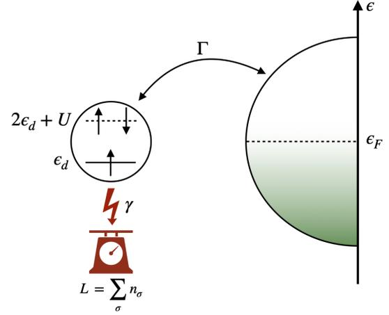
FIG. 1. Sketch of the setup for the Kondo-Zeno Crossover. A singly-occupied quantum dot is coupled to a large metallic bath via a hybridization  $\Gamma$  and to a measurement apparatus continuously monitoring, with rate  $\gamma$ , its total charge. Upon averaging over the monitoring noise the dynamics of the dot plus metallic bath is described by Lindblad master equation with a jump operator  $L = \sum_{\sigma} n_{\sigma}$ , describing charge dephasing.
