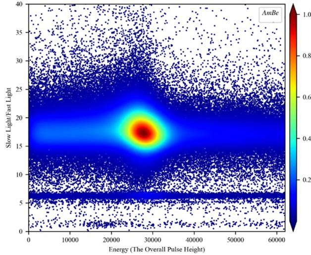
Figure 2. Scatter density plot of the signals captured by the detection system exposed to Am-Be Neutron source.
