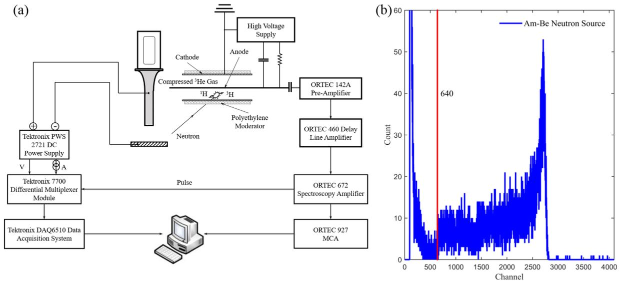
Figure 4. Helium-3 proportional counter based neutron detection system (a). Schematics of the  $^3\text{He}$  neutron detection system (b). Detected differential pulse height spectrum when exposed to an Am-Be neutron source.
