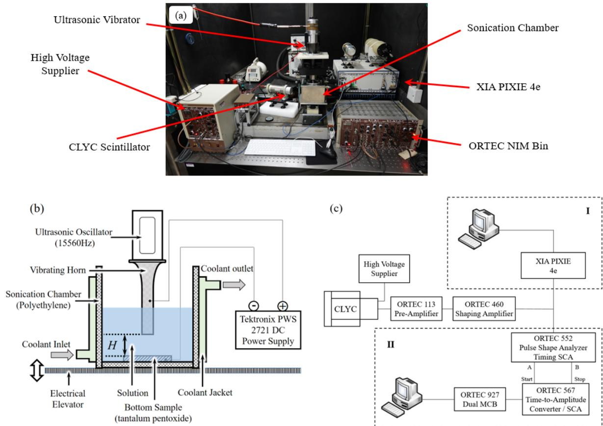
Figure 1. Experimental Setup (a). Arrangement of sonication platform and neutron detection system. (b). Schematics of sonication chamber. (c). Logic circuit diagram of neutron detection system.
