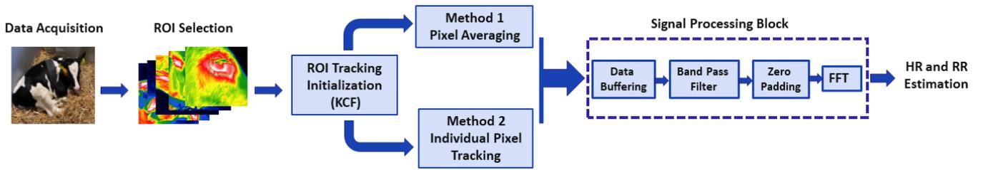
Fig. 1: Block diagram illustrating the process flow for estimating heart rate and respiration rate from thermal images of calves.
