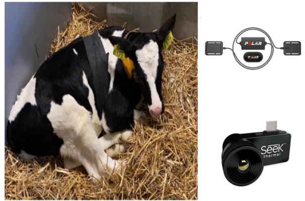
Fig. 3: A calf with a heart rate sensor, the Seek Thermal camera, and the Polar Electrode Set used in the study.
