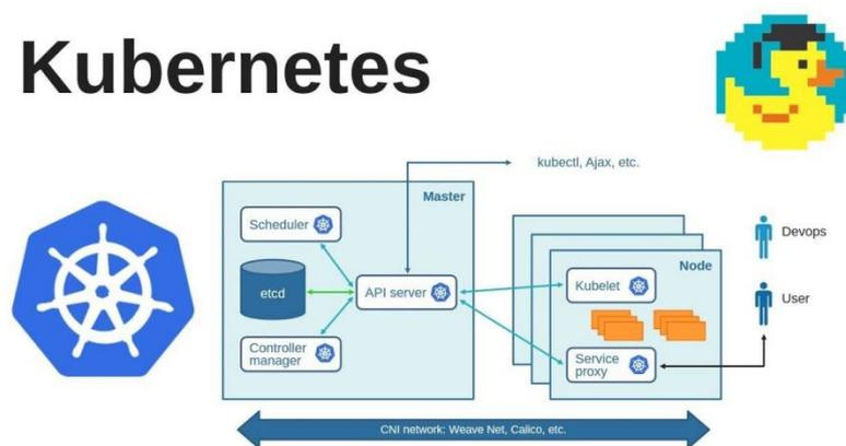
**Figure 4.** Kubernetes (K8s) automated deployment environment architecture
