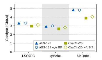
Fig. 4: Impact of header protection for different AEAD algorithms and QUIC implementations on the goodput.
