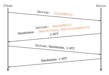
Fig. 1: Simplified illustration of a QUIC 1-RTT handshake.
