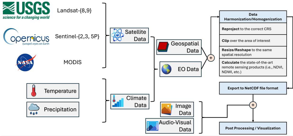
Figure 2: The workflow architecture of the Ocean-DC implementation.
