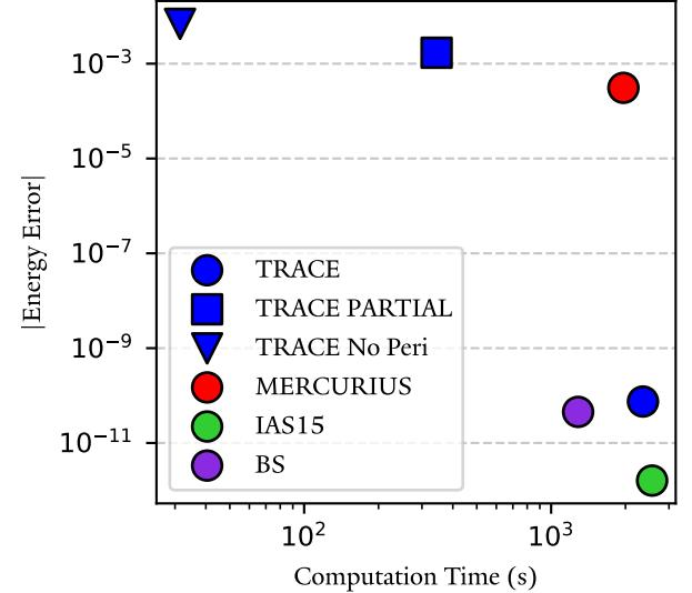
**Figure 6.** Efficiency plot of various integrators for the large- $N$  accretion problem without considering collisions. TRACE, BS and IAS15 all perform very well from an error standpoint, but are quite slow. MERCURIUS is just as slow, but is far less accurate. TRACE Partial and TRACE no Peri offer much fast alternatives while maintaining roughly the accuracy of MERCURIUS.
