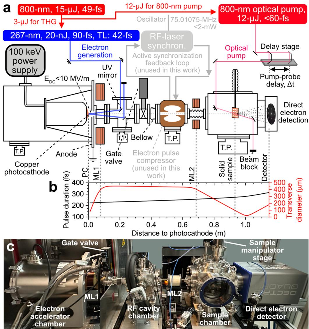
**FIG. 3.** (a) Schematic of the 30 kHz, 95 keV HiRep-UED instrument, with each component labelled. See main text for more details. (b) General Particle Tracer (GPT) simulation of the electron pulse duration (blue distribution) and transverse diameter (red distribution) with the instrument operating in the temporally uncompressed mode using an electron beam containing 55 electrons. All values are given in FWHM. (c) Image of the instrument in the laboratory.
