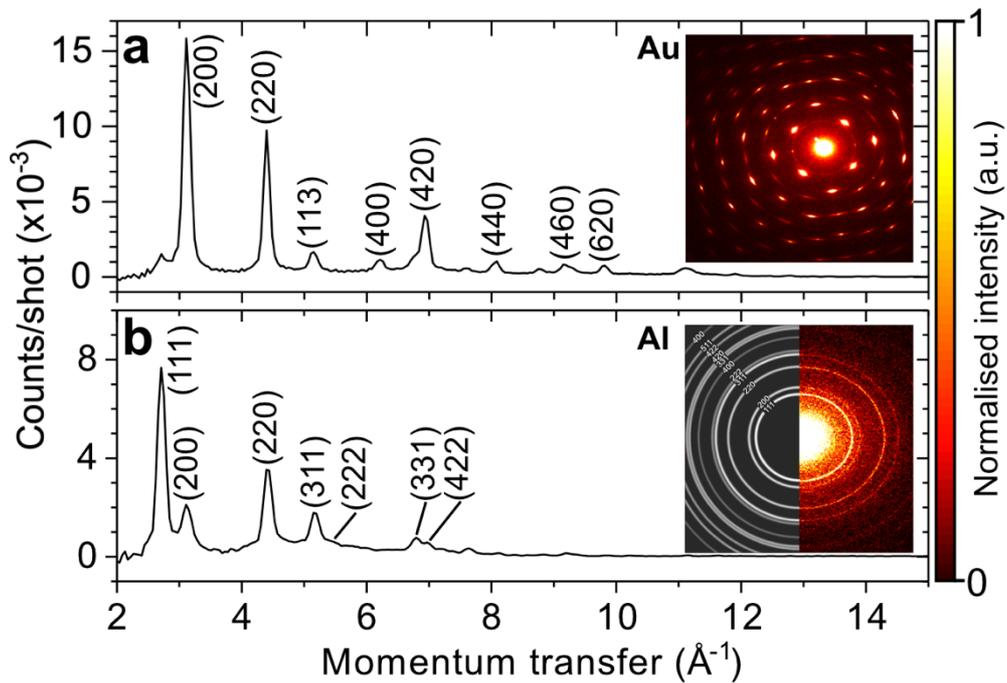
**FIG. 5. (a-b)** Electron diffraction patterns of (a) 11-nm monocrystalline gold (Au) and (b) 31-nm polycrystalline aluminium (Al) measured using a 95-keV electron pulse containing  $\sim 100$  at 30-kHz with a direct electron detector. Both data were measured without apertures. Insets: measured detector images, with simulated data shown for aluminium.
