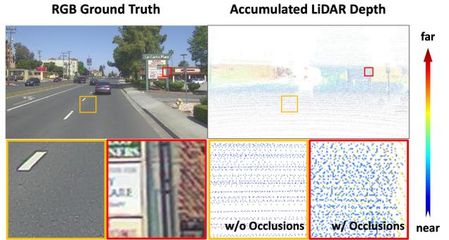
Figure 3. **Illustration of the occlusion issue on the depth map projected from accumulated Lidar points.** Observe that multiple layers of surface points may project to the same region on the image, yielding ghost depth points.
