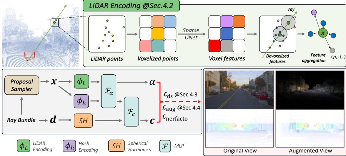
Figure 2. **Overview of LidarRF** – it takes as input the sampled 3D positions  $\mathbf{x}$  and ray directions  $\mathbf{d}$ , and outputs corresponding density  $\alpha$  and color  $\mathbf{c}$ . It incorporates both hash encoding and LiDAR encoding using a sparse UNet. Additionally, augmented training data is generated through LiDAR projections, and the geometry prediction is trained with our proposed robust depth supervision scheme.
