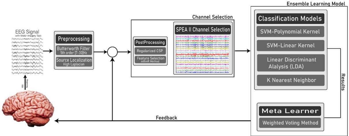
Figure 1: Diagram illustrating the Proposed Channel Selection Method
