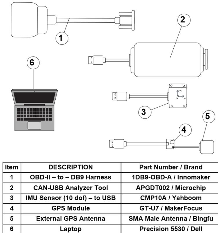
**Figure 1.** Automotive CAN reverse engineering kit (modified from [8]).
