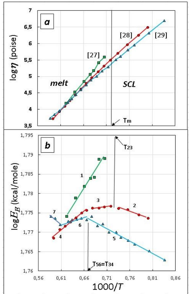
**Figure 4.** Experimental viscosity-temperature data for  $GeO_2$  after *de Neufville et al* [27, Pt viscometer] (line 1), *Fontana & Plummer* [28, Run 1] (lines 2-4), and *Bruckner* [29] (lines 5-7) presented in the *Arrhenius* plot (a) and in the *TA*-plot (b).
