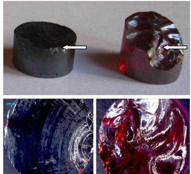
**Figure 9.** The fractured samples of “magnetic” (on the left) and “non-magnetic” (on the right) As<sub>2</sub>S<sub>3</sub> glasses; a sight from sideways (top) and from above (bottom).
