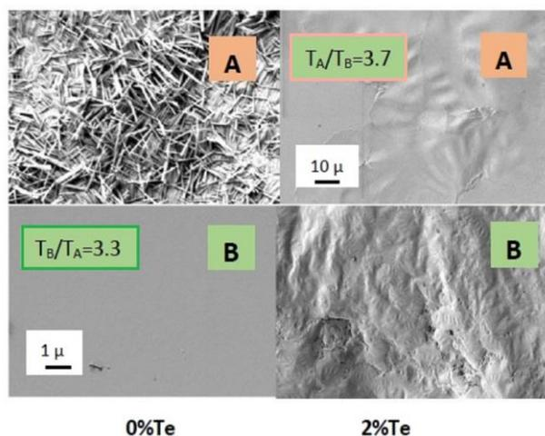
**Figure 11.** The SEM images for two final Se-Te samples fractured along (A) and across (B) the US input (see **Fig.10**).
