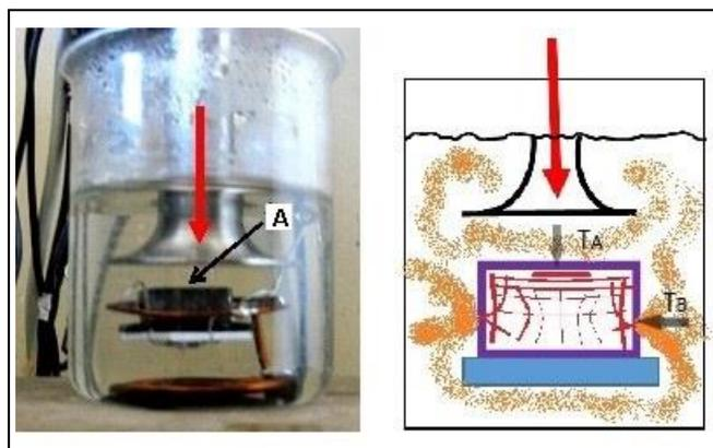
**Figure 10.** US-treatment of Se-X samples: the cell (on the left) and the scheme of action (on the right). Red arrow is the US input, red curves are the wavefront section. Arrows  $T_A$  and  $T_B$  indicate two directions for measurement of optical spectra.
