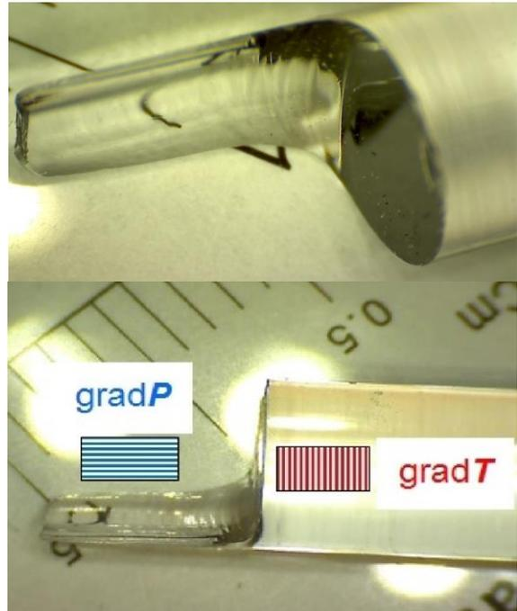
**Figure 8.** The frozen wavefronts of two bond waves directed previously by the temperature and pressure gradients.
