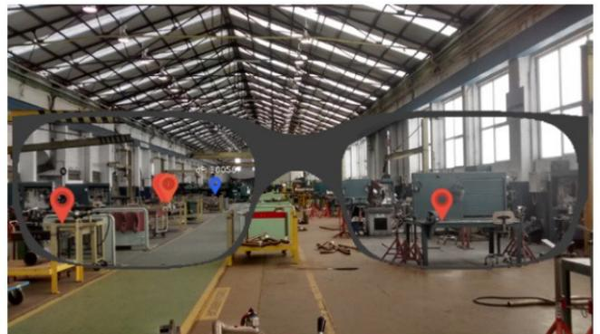
FIGURE 4: Localization of products inside a workshop using an IAR system.
