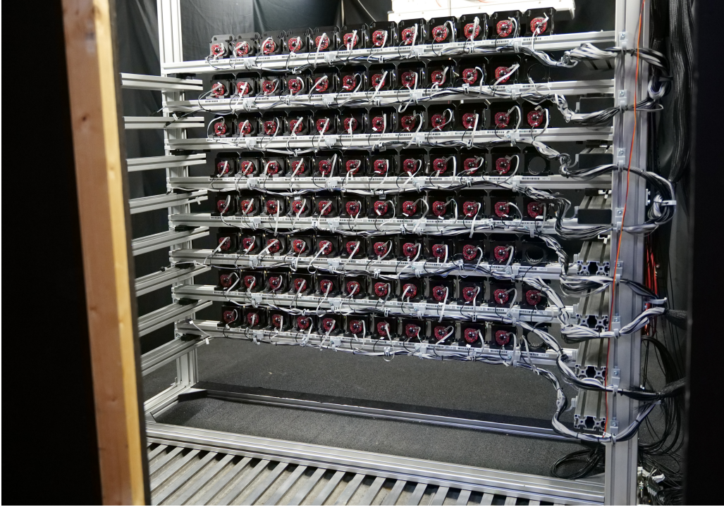
Figure 4. Backside of the PMT rack inside the testing facility. Each PMT is connected to an mDOM mainboard with a coaxial and ribbon cable. Each PMT position is marked with a barcode.
