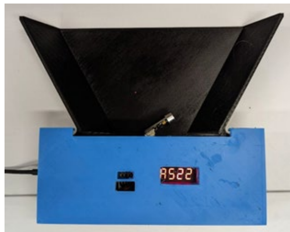
Figure 6: Actual Conical structure containing the CMOD A7 and microphone.
