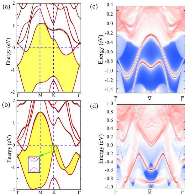
FIG. 6: Band structures for (a)  $H_1$ - and (b)  $H_3$ - $Nb_2NF_2$  without (black) and with (red) the SOC. The full-gap near the Fermi level for both structures with SOC are decorated by yellow. Edge states of the corresponding semi-infinite slab for (c)  $H_1$ - and (d)  $H_3$ - $Nb_2NF_2$ .
