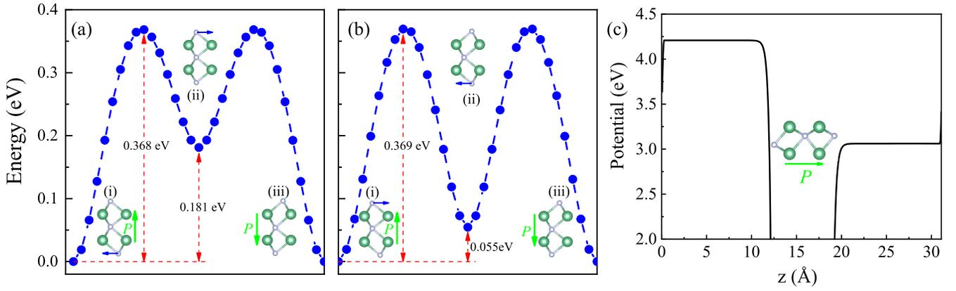
FIG. 3: NEB calculations for polarization direction reversal in  $\text{H}_3\text{-Nb}_2\text{NF}_2$ , considering (a) the  $\text{H}_1$  and (b) the  $\text{H}_2$  non-polar  $\text{Nb}_2\text{NF}_2$  as intermediate state. The polarization direction is indicated by the green arrow accompanied by the symbol P. (c) The averaged electrostatic potential of  $\text{H}_3\text{-Nb}_2\text{NF}_2$  in the out-of-plane direction.
