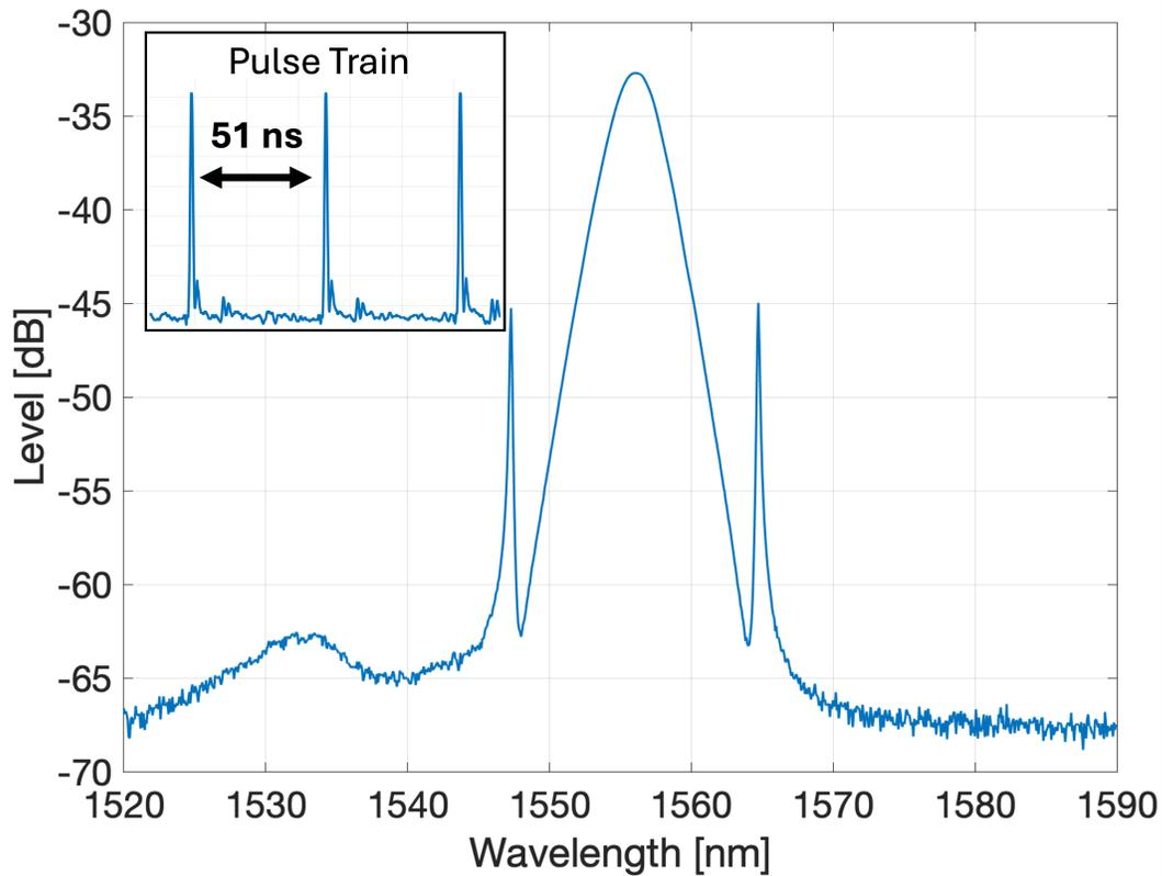
Figure 5: Fundamental modelocking spectrum at room temperature. Inset: pulse train.
