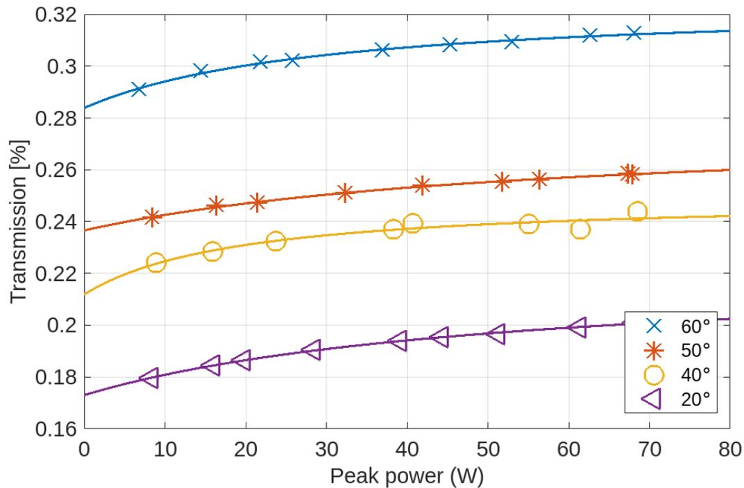
Figure 3: Transmission through SWCNT/PDMS coated tapered fiber as a function of peak power.
