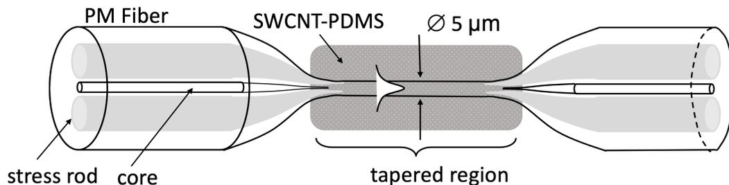
Figure 1: (a) PM tapered fiber device with SWCNT/PDMS composite.
