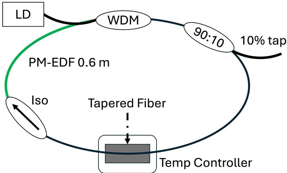
Figure 4: Set-up of mode-locked fiber laser with SWCNT/PDMS saturable absorber. LD - laser diode, WDM - wavelength division multiplexer, Iso - isolator, EDF - erbium doped fiber.
