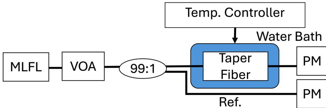
Figure 2: Set-up used to measure the saturable absorption of SWCNT/PDMS coated tapered fiber at varying temperatures. MLFL - modelocked fiber laser, VOA - variable optical attenuator.
