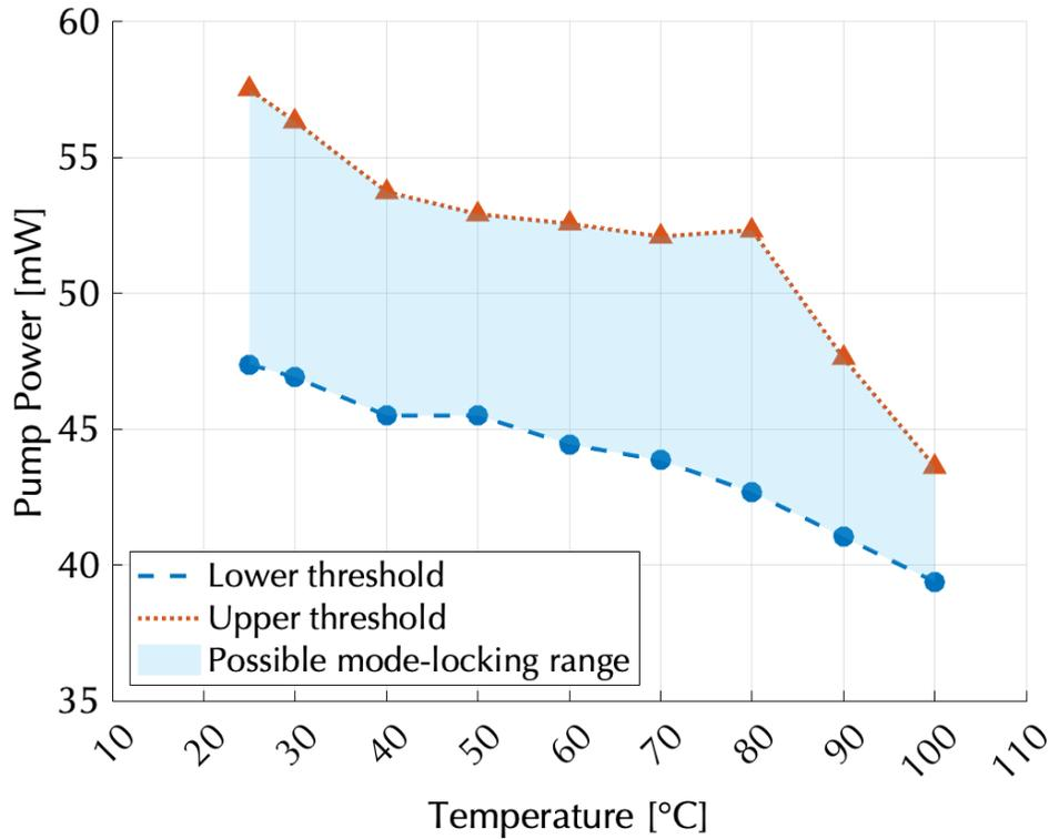
Figure 6: Possible range of pump power for fundamental modelocking.
