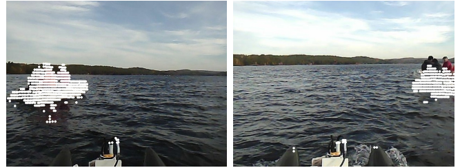
Fig. 14: Alignment (left) and misalignment (right) of fused sensors (LiDAR and RGB camera) due to the ego- and obstacle-motion on the water, despite the same calibration parameters.
