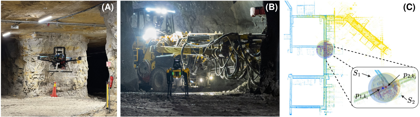
Fig. 1: (A) One of the custom-built quad rotors that was utilized during the series of experiments in this article. (B) Spot in a construction area during the field trials. (Copyright NCC) (C) The outcome of the proposed framework from a larger scale indoor environment from Luleå University of Technology, where the two robots start together but explore different branches of the building.
