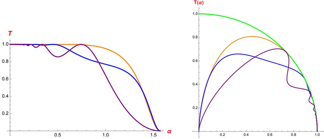
Figure 15: Transmission coefficients  $T(\alpha)$  of electric wells for  $k = 1$  as a function of  $\alpha$  and for three depth values of the well:  $v_0 = 8$  (purple),  $v_0 = 1$  (in blue),  $v_0 = 1/8$  (orange).
