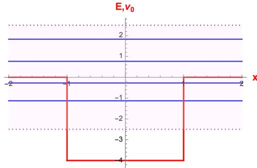
Figure 18: Spectrum of the electric waveguide for  $v_0 = 4$  and  $k = 2.5$  corresponding to the magenta line of Fig. 17.
