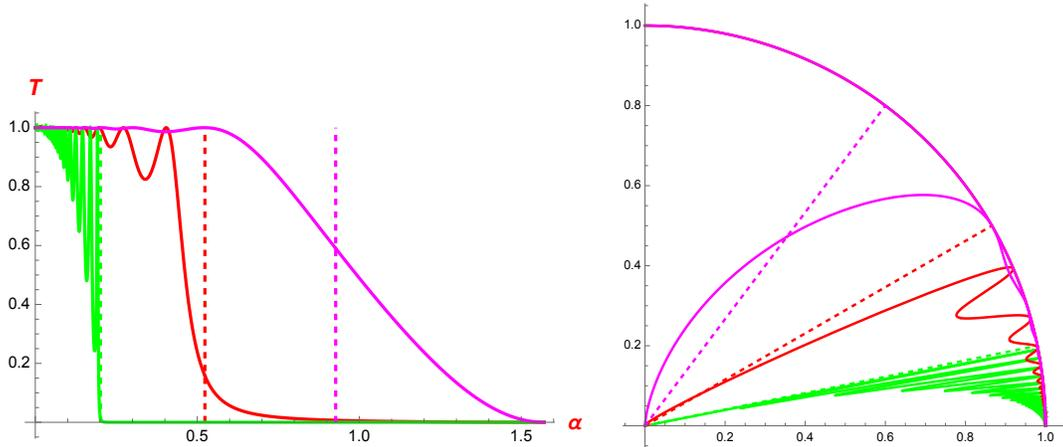
Figure 8: (left) Transmission coefficients for  $k = 1$  and different values of the well depth:  $a_0 = 4$  (green),  $a_0 = 1$  (in red),  $a_0 = 1/4$  (magenta). (right) The same results in a circular plot of the transmission coefficient  $T$  versus the angle of incidence  $\alpha$ . The dashed radius (or vertical lines in the left graphic) correspond to the limit of allowed/not allowed classical scattering given by formula (3.14).
