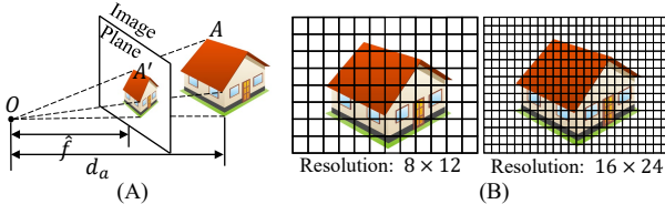
Fig. 6 – Pinhole camera model. (A) Object A positioned at a distance d_a undergoes projection onto the image plane. (B) Employing two cameras for capturing an image of the car. The left one has a larger pixel size. Although the projected imaging sizes are the same, the pixel-represented images (resolution) are different.
