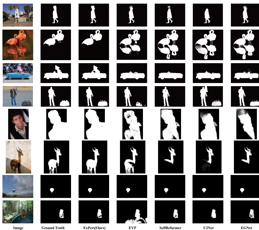
Fig. 5: The qualitative results of ExPert and four SOTA models. From left to right are the images, the ground truths, ExPert’s masks, EVP’s masks, SelfReformer’s masks, U2Net’s masks and EGNet’s masks. Better visual effect when zooming in.
