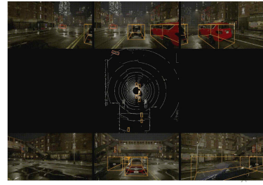
Fig. 7. 3D object detection by ContextualFusion on AdverseOp3D (CARLA generated) data at night while raining
