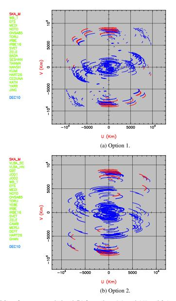
Fig. 4: Map of uv coverage in band C1 for options 1 (panel (a)) and 2 (panel (b)), with target sources' Decl. (J2000) =  $10^{\circ}$ . The uv coverage was mapped with the tool provided at http://www.aoc.nrao.edu/software/sched/.
