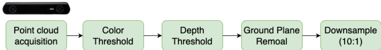
Figure 5: Schematic for point cloud segmentation and downsampling process used in the study
