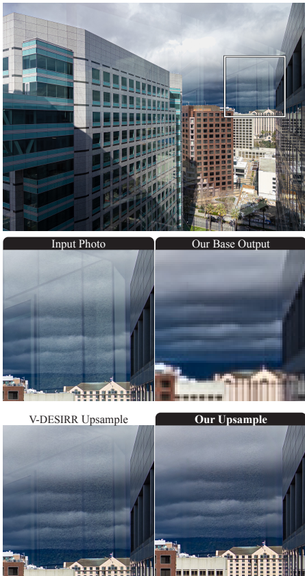
Fig. A9: Upsampling high frequency texture. V-DESIRR [36] re-introduces reflections that were removed at 256^2 pixels. Our method removes these, but textures that were not visible at 256^2 are copied.
