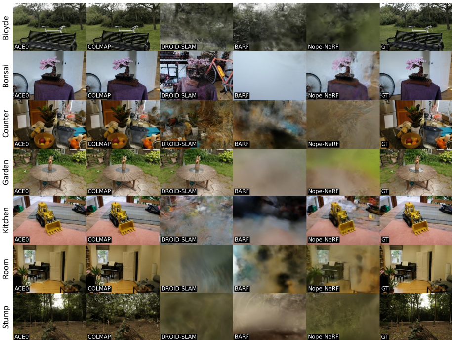
Fig. 10: View Synthesis Quality on the MIP-NeRF 360 dataset. For each scene, we show the test image where ACE0 achieves its median PSNR value. For comparison, we show the corresponding results of our baselines as well as the true test image (GT). These results correspond to Table 2 (b) .
