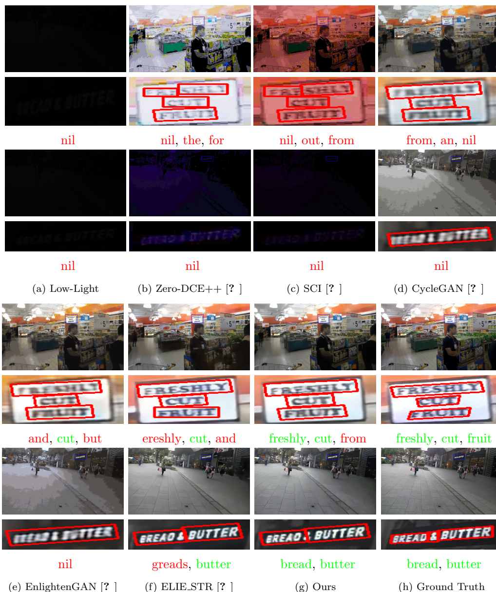
Figure 5: Comparison of our model with other state-of-the-art methods on the Syn-IC15-Fuji-v1 (top) and Syn-IC15-Fuji-v2 (bottom) datasets. PAN [? ] is used as the text detector, while ASTER [? ] is used for text recognition. Blue boxes represent the zoomed-in regions, while red boxes are drawn based on the predictions of PAN. Text recognition is performed on the word images cropped by using PAN’s predictions (from column 5a to column 5g) and ground truth text boxes (column 5h). “nil” stands for either no recognition results or invalid prediction boxes (with \text{IoU} \leq 0.5 ) which are not considered for the subsequent recognition.
